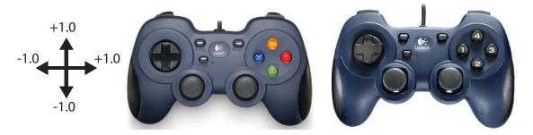
getStickHL() or stick.horizL() or stick.horiz() [returns double.] Returns a number between -1.0 and +1.0 indicating how much the left thumbstick is displaced horizontally. As indicated in the figure above, a value of -1.0 corresponds to the stick all the way to the left. A value of +1.0 corresponds to the stick all the way to the right. When the stick is released and allowed to return to the center, it returns a value of 0.0.
