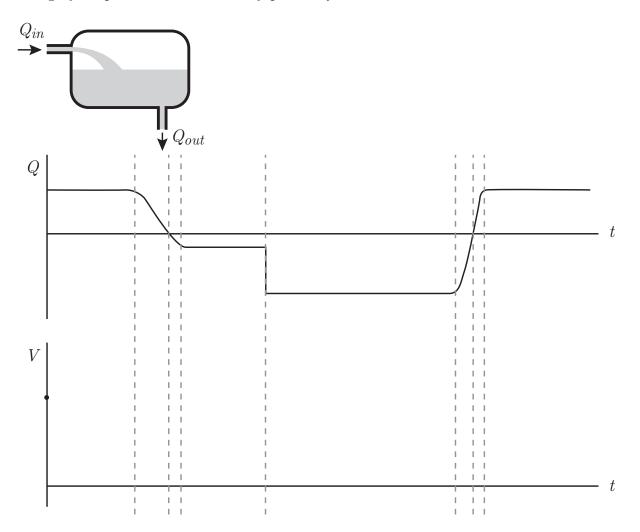
Now, let's do the reverse operation. Suppose you are given the volume of water V as a function of time as shown in the top plot. Given this, generate the plot of the net flow rate, Q, as a function of time.
